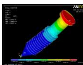
Fig.11. The displacement distribution on the implant-bone interface when the titled angle is 60°
